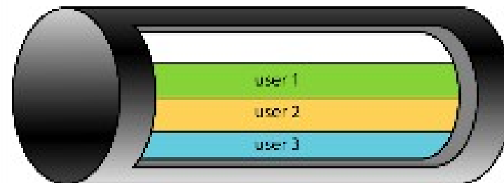
Figure 6 - Shared traffic ensures each user receives a fair share of the available bandwidth
